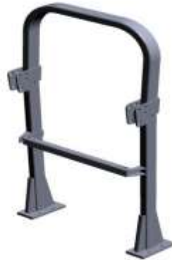
Figure 2: CAD model of two post foldable ROPS.
